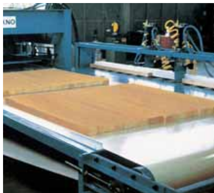
Manufacture of wood core plywood boards.
